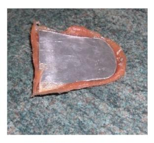
Usind a dremol, flapwheel on a drill, a file or glass paper remove all the surplus P40 flush with the top of the alloy plate and flush with the back of the plate and the edge of the nozzle. If there are are any gaps on the edges it will pay you to try again, however you can use the shoe you have made to improve your template shape
