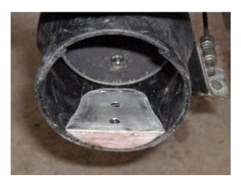
Make sure that the pump casting doesn't land ontop of the shoe and reduce the amount of trim you have. Put the washers and nut on the bolts ( dont forget to use some thread lock or nyloc nuts)
